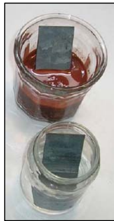
Figure 3. Comparative corrosion testing between saturated hematite and de-mineralised water
